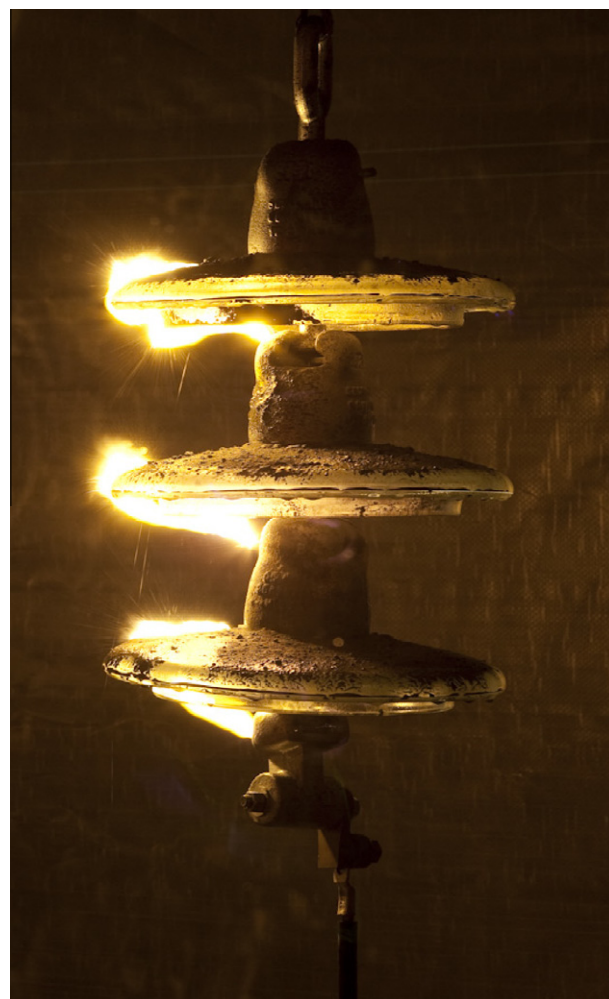
Fig. 5. An example of a flashover (three faults) on a glass string insulator. The insulator has been coated with 3 mm of wet volcanic ash. Flashover occurred at ~40 kV (insulator string design voltage 40 kV).
